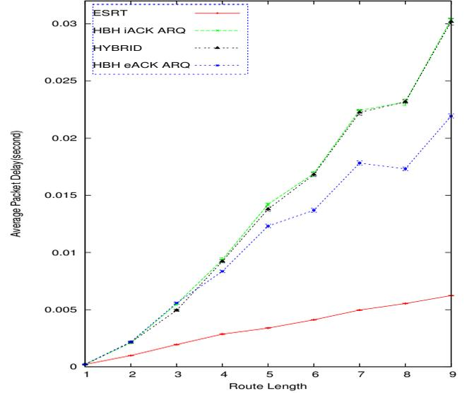
Fig. 8. Average packet delay for  $p = 0.20$ .
