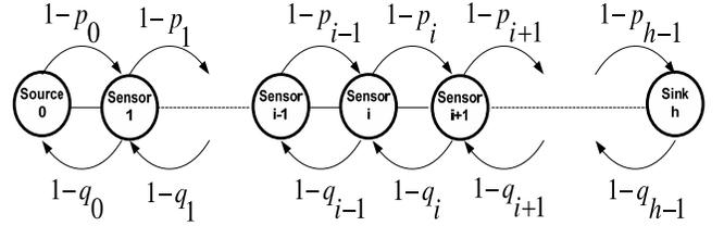
Fig. 1. A single route with transmission failure probabilities.
