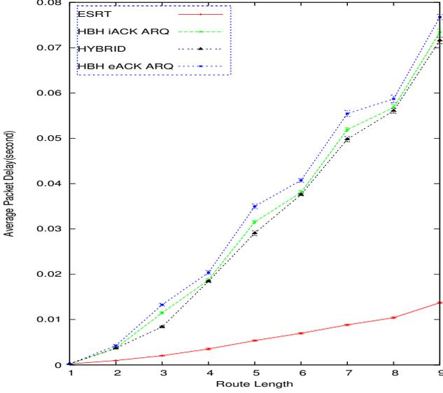
Fig. 9. Average packet delay for  $p = 0.45$ .
